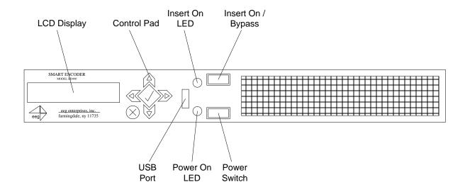
**Power Switch** This is the on/off switch for the unit.
